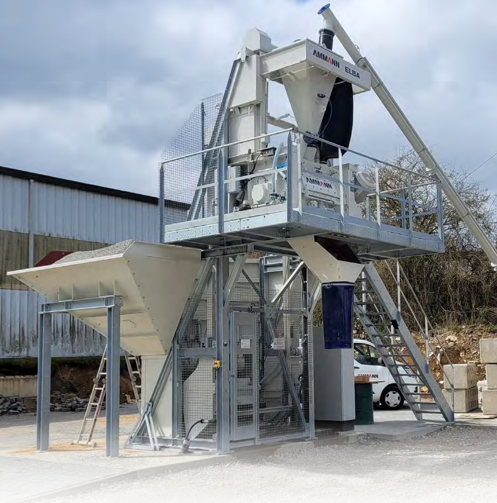
Overview of the newly installed Ammann CFS 30 SL Elba ready-mix concrete plant from A. Heßler. The plant is flexibly designed, allows special mixtures, and offers filling options for large and small concrete quantities.
