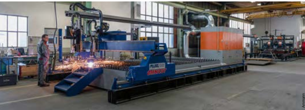
The plasma machine is used to cut Amdurit plates to size. It is then used for mechanical post-processing in the form of drilling, counter-drilling and tapping.
