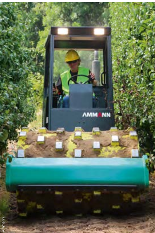
A new application for lightweight single drum rollers was found in the compaction of access and connection tracks in fruit orchards.
