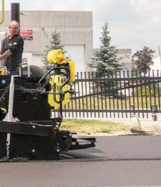
Pavers and in particular their screeds are of pivotal importance to the quality of the road surface. All the more important, then, to explain in detail how these complex machines work during the training event.
