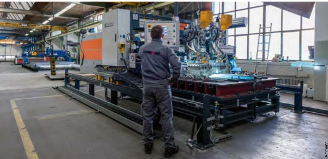
The Amdurit production lane at the Ammann Group’s headquarters in Switzerland. Everything is handled by a single process – from build-up welding (in the foreground), to cutting and mechanical processing, to forming on a steel press.
