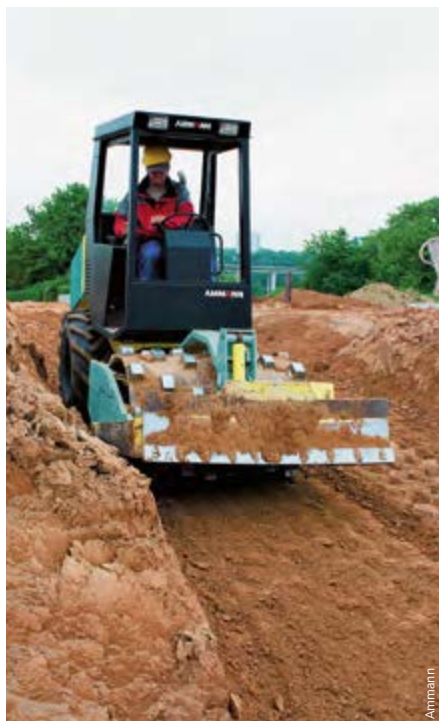
The sister machine of the ASC 50: an ASC 30 with dozer blade.
